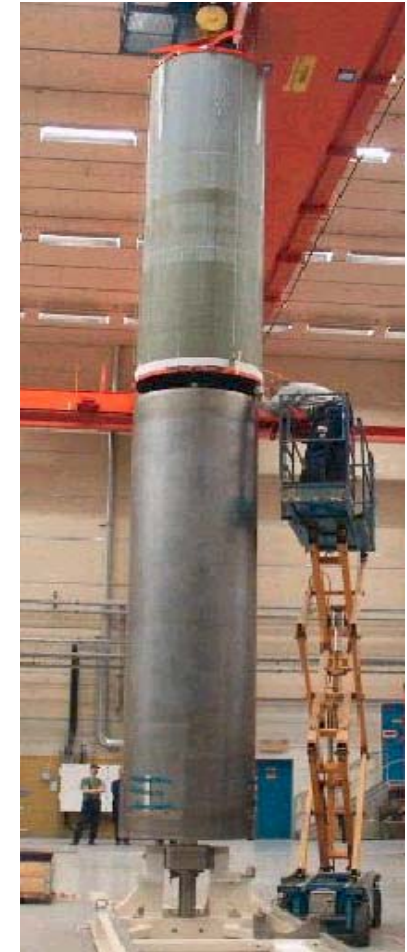
Qual model of the Spacebus central tube and central tube during demoulding (courtesy Saab Ericsson Space)
