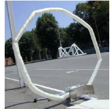
epoxy resin glass fibers UV curing (Astrium-SAS France)
