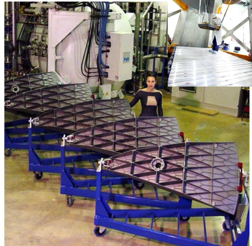
Petals of Herschel telescope SiC 100
