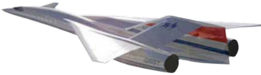
Figure 16: Supersonic Aerospace International's Quiet SST may have solved the sonic boom problem through the shape of its fuselage. Futuristic superconductive energy storage and electrically driven turbofans based on a design first developed by Henri Coanda in 1910 could be the precursor of petroleum-free flight (Courtesy of EV world)
