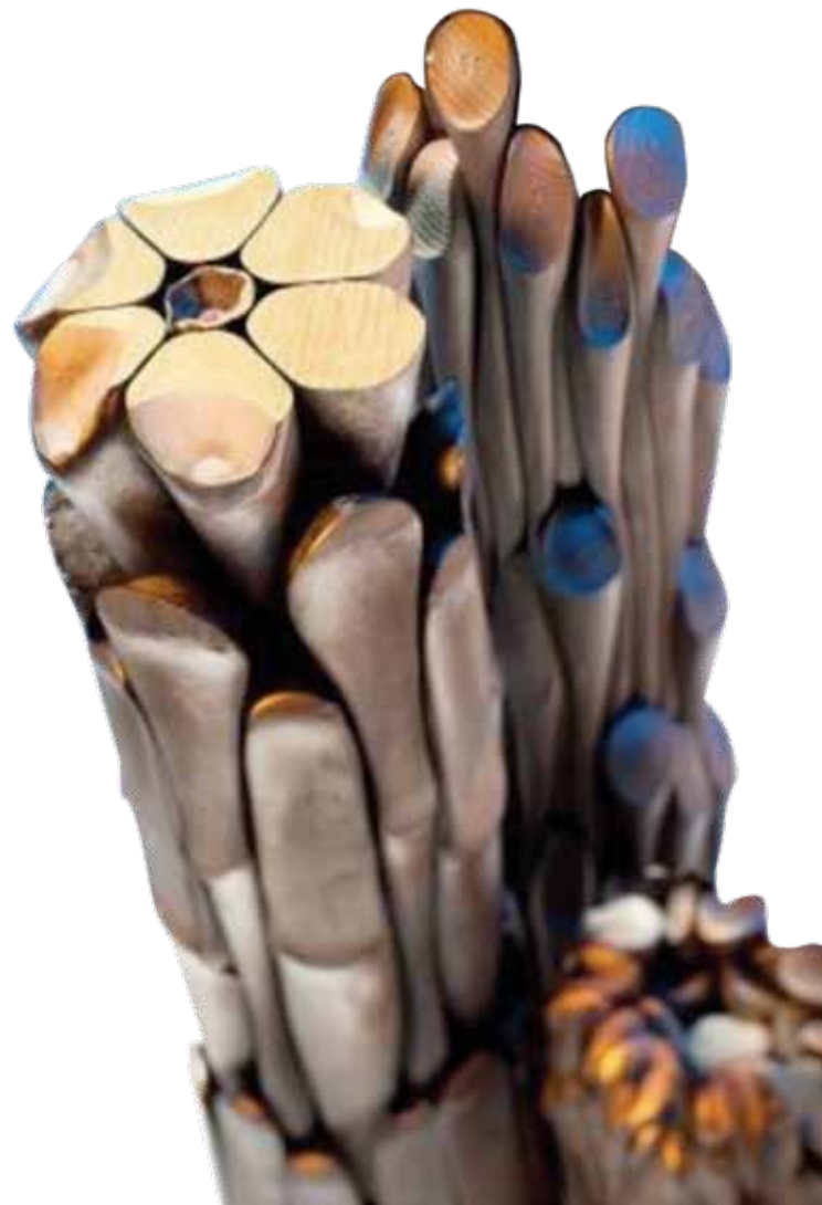
Figure 4: Superconducting billet before processing to long thin wires.
