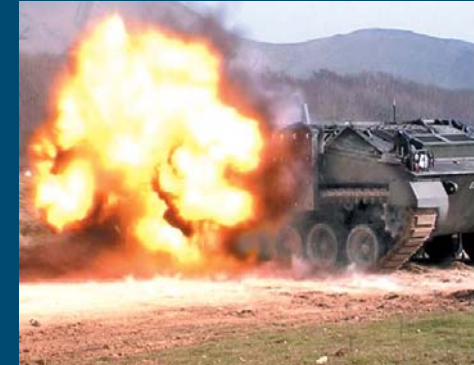
Electric armour test against rocket propelled grenades
