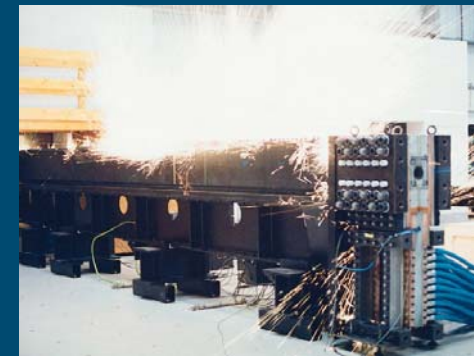
90mm electromagnetic gun test firing
