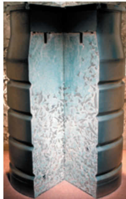
Cut-away view of an intermediate level waste container
