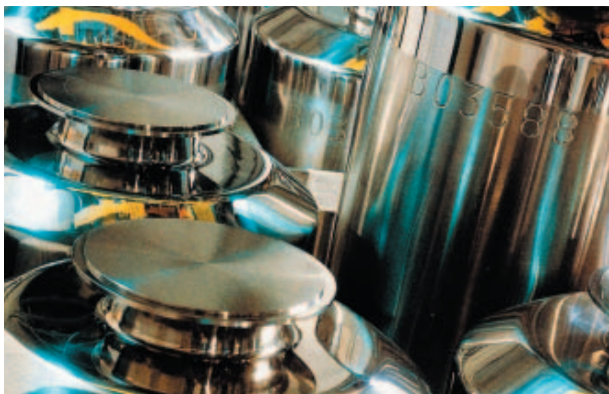
High level waste containers. [Courtesy of Nexia Solutions].
