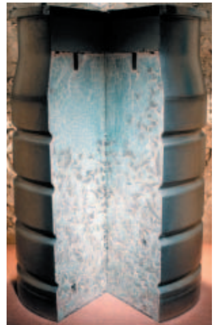
Cut-away view of an intermediate level waste container
